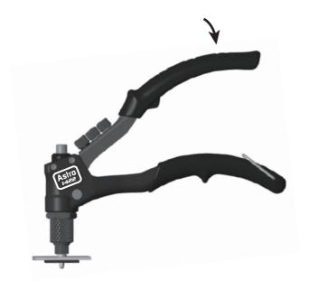
4. After setting the rivet in the work piece, release handles in the open position. It may take several pumps to set your rivet. Tilt the tool backwards after the rivet pops to expel the rivet stem from the rear of the tool.
