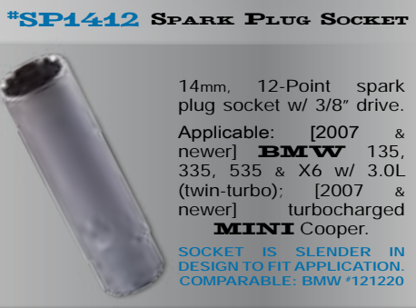
*SP1412 SPARK PLUG SOCKET
