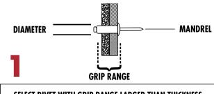
SELECT RIVET WITH GRIP RANGE LARGER THAN THICKNESS OF MATERIALS TO BE FASTENED. DRILL HOLE SAME SIZE AS RIVET DIAMETER.
