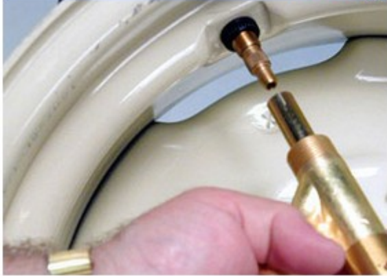
The sleeve is split to slide over the core housing.
