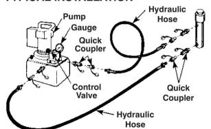
A double-acting cylinder or ram can be either extended or retracted hydraulically.
