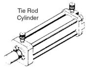
NOTE: The capacity of a hydraulic system is determined by the effective area of the cylinder and the system pressure.
