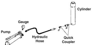
Since the single-acting cylinders have only one hose going to the cylinder, the cylinder can only apply force to extend (pull cylinders retract) its rod. The return stroke is accomplished by gravity or spring force.
