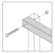
Attach horizontal posts with the supplied nuts and bolts.
