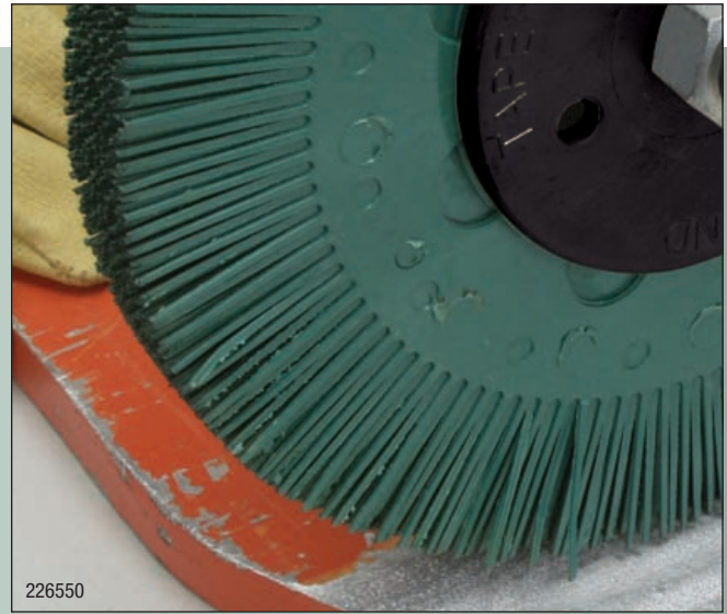
8" Radial Bristle Brush, grade 50, removing paint mounted on a straight shaft tool.
