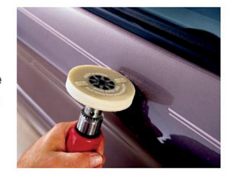
Remove vinyl stripes, numbers, letters and graphics from gel coat and painted marine surfaces without damaging the finish
