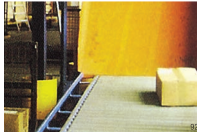
Corrugated boxes slide more easily down a chute lined with abrasion-resistant 3M™ UHMW-PE Tapes.
