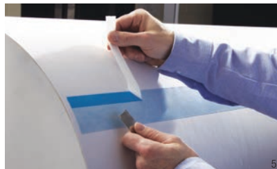
One simple splice with 3M™ Splittable Flying Splice Tape replaces complex patterns.
