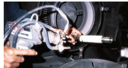
For thermal spray and plasma spray masking, 3M™ Glass Cloth Tape 361 with silicone adhesive performs reliably at up to 450°F (232°C). Passes FAA flame resistance regulations.
