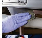
**Surface Prep Hand**Sand edges and other hard to reach areas using P400 flexible abrasive sheet or Scotch-Brite™ Hand Pad until the surface is matte and all sheen has been removed.
