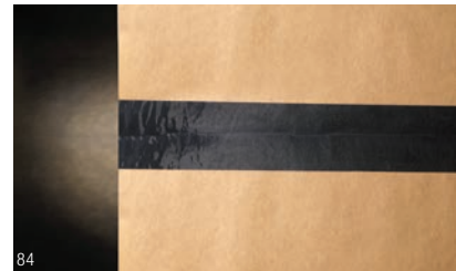
For marking splice location, 3M™ Polyester Tape 850 is available in red, black, white and silver. Transparent is also available to blend with the web stock. Pressure sensitive acrylic adhesive grabs on contact and holds butt splices securely. High tensile strength backing resists web handling stresses.
