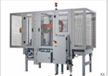
800rf* Up to 10 cs/min Up to 65 lbs Side belt drives
