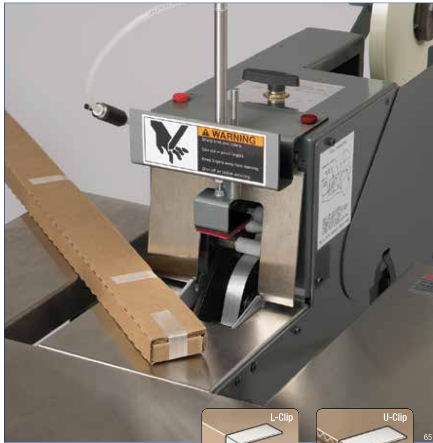
3M-Matic™ L-Clip Applicator S867 with optional U-Clip adapter.
