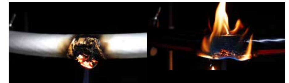
Cable Protected with Scotch® Fire Retardant Electric Arc Proofing Tape 77 During Test
