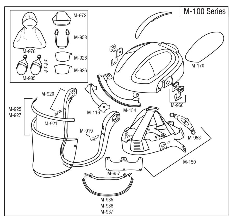
If you discover any signs of wear and/or damage, remove headgear from use and service or replace as appropriate. 3M recommends a maximum life (shelf life plus in use life) of 3 years from the date of manufacture. See the M-Series User Instructions for details on inspection and replacement.
