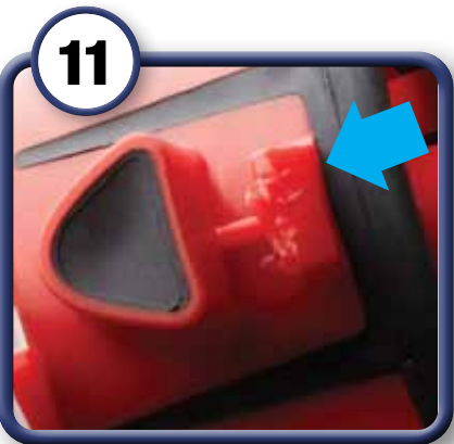
Inspect atomizing head for damage or wear which could result in fluid leaks or poor performance.
