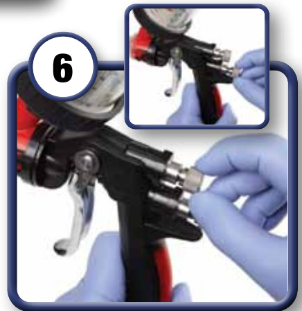
Adjust fan and fluid flow to achieve the desired size and wetness of the pattern. NOTE: when closing the fan adjustment completely it may be necessary to re-adjust the air flow control valve.
