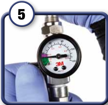
Set air pressure at 15 psi for 2 nd stage (air and fluid flowing)
