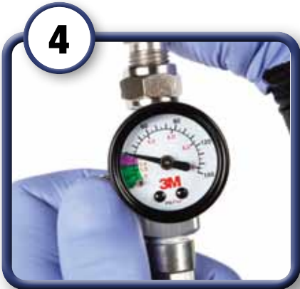
Set air pressure at 25 psi for 1 st stage (only air flowing)
