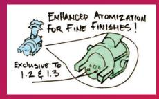
We added extra atomizing air holes to the new 1.2 mm and 1.3 mm atomizing heads to ensure you're getting the premium performance you expect out of your metal guns, while making cleaning quick and easy with see through atomizing heads.
