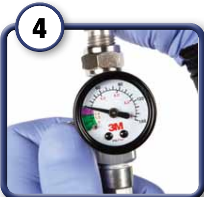
4 Set air pressure at 25 psi for 1 st stage (only air flowing)
