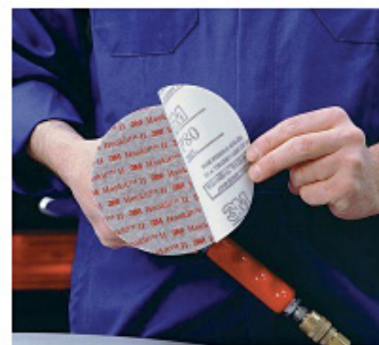
Hookit™ discs both apply to the pad and peel away with ease.
