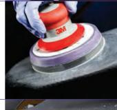
**Surface Prep Machine**Sand remaining surfaces using P400 abrasive on a DA sander until the surface is matte and all sheen has been removed. Note: Use 3M™ Hookit™ Hard E-coat Disc on hard to sand aftermarket parts.
