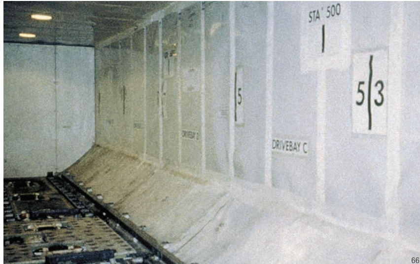
For seaming and sealing panels in aircraft cargo bays, 3M™ Glass Cloth Tape 398FR exceeds flame retardant standards F.A.R. 25.853 (a) and F.A.R. 25.855 (d). Pressure sensitive acrylic adhesive bonds on contact to many surfaces. High adhesion is secure for extended periods. Rugged cloth surface resists wear from heavy bags.
