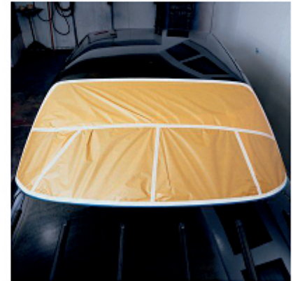
Excellent resistance to bleed through makes this masking paper ideal for windshields
