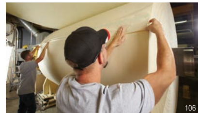
For finished mill overlap splicing, 3M™ Repulpable Permanent Tape provides high shear strength without adhesive oozing or bleed through.
