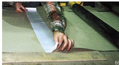
With high tensile strength and rubber adhesive, 3M™ Glass Cloth Tape 365 reliably splices fabrics and other textured surfaces.
