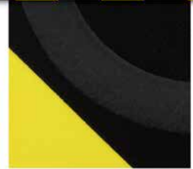
3M™ Safety Stripe Tape 5702 After 1,000 abrasion wear cycles, the black color is still visible.
