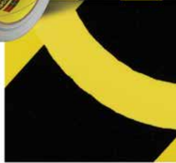
Competitive Safety Stripe Tape After 1,000 abrasion wear cycles, the color black is worn away.
