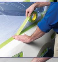
**Overspray Protection**Ensure that the car is completely dry prior to applying plastic sheeting. Mask entire vehicle with plastic sheeting. Cut out the repair area with a razor blade. Tape the plastic sheeting directly to critical masking edge.
