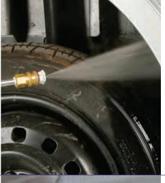
**Pre-Cleaning**Pre-wash/clean vehicle prior to disassembly (power wash undercarriage area at repair).
