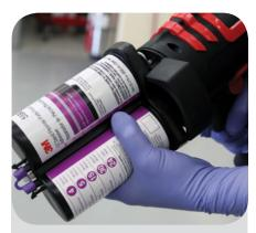
**TWIST** a cartridge into place on the applicator until it locks into place.
